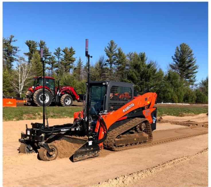
Accuracy in the level of the sand is essential. The EG1 Laser Grade Control System provides accurate grading results in less time with less labor. The system is versatile, efficient, economical and durable and can be used for numerous applications including field grading, lot leveling, laser screed and automated control.
