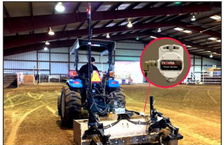
EG2-S on a tractor pulled box blade
